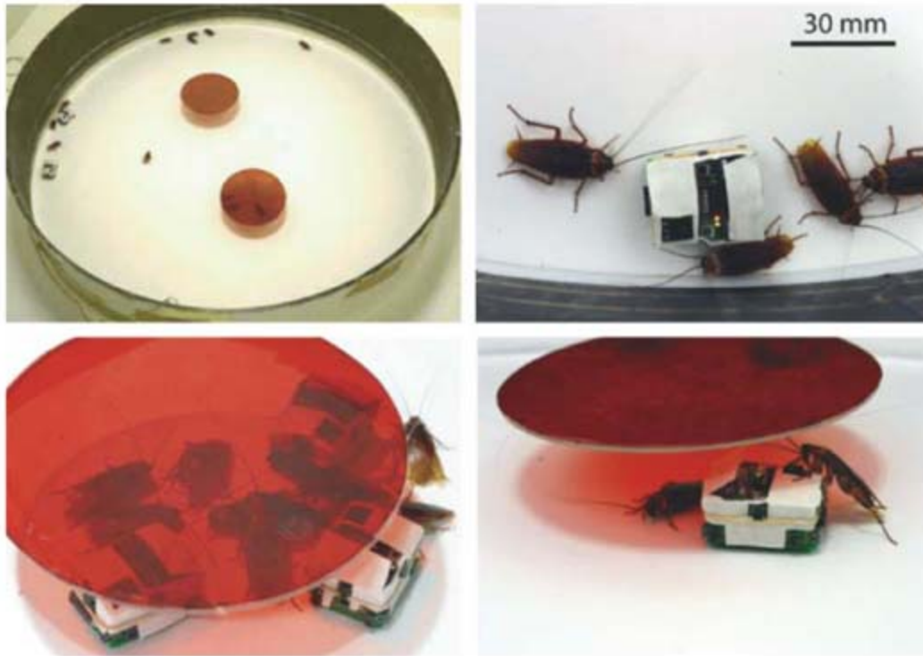
Fig. 1. Experimental setup showing the cockroaches ( Periplaneta americana ) and the robots. Two shelters (150 mm) made of plastic disks covered by red film filters are suspended (30 mm) above the floor of a circular arena (diameter 1 m). The darkness under the shelter is controlled by the number of layers of red film. Cockroaches aggregate under the shelters (18).
